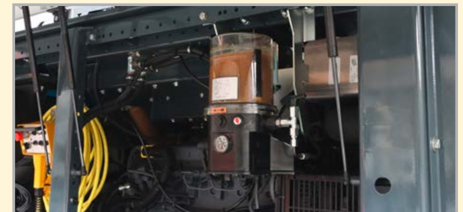
The electric central lubrication system saves time and minimizes wear
