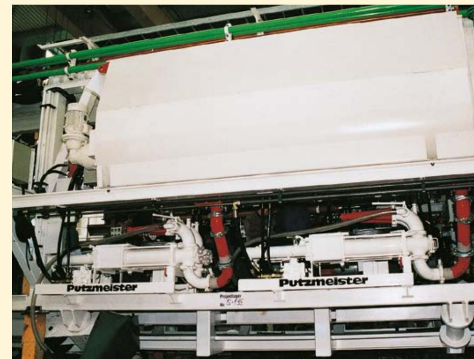
Space-saving installation of two KOV 550 DUO underneath a 6 m<sup>3</sup> agitating trough
