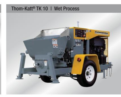
This proven pump fills the void between small-line mechanical ball valve pumps and 5–6 in (127–152mm) cylinder-diameter concrete pumps. The swing-tube design gives operators the benefit of reversing to relieve pressure due to plugs, pumping difficult low-slump or fiber mixes and lower maintenance costs. The 3-inch (76mm) material cylinders and variable, smooth hydraulics allow extremely controlled low output for specialized applications.
