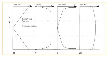
Fig. 26: Flow influences on the pipe conveying of fresh concrete a) Shear stress b) Viscosity c) Shear speed d) Speed profile
