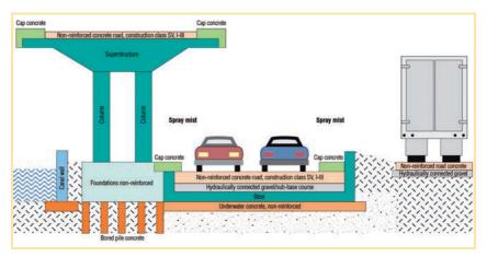
Fig. 15: Exposition classes in the engineering construction\*
