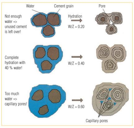
Fig. 2: Diagram showing the reaction of cement and water (hydration)
