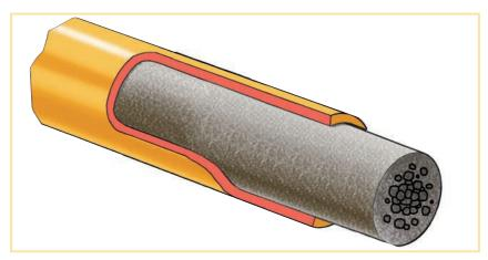
Fig. 27: Schematic representation of boundary zone segregation
