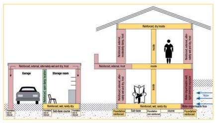
Fig. 13: Exposition classes in the residential construction\*
