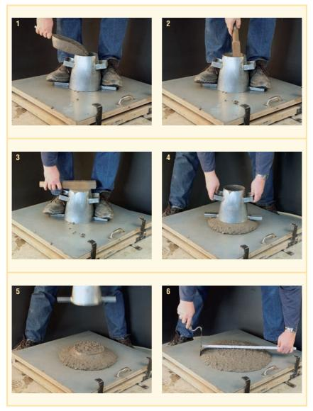
Fig. 10: Measuring spread in accordance with DIN EN 12350-5
