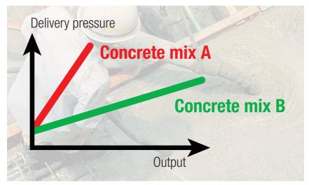
Fig. 35: Effect of different concrete recipes on pumping
