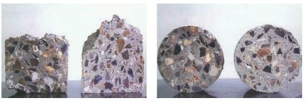
Fig. 25: Radial cross-section through the stream of concrete, left = blockage, right = flowing\*
