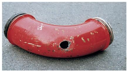
Fig. 31: Pipe wear in the delivery line bend
