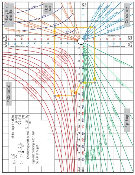
Fig. 33: Concrete pressure performance nomogram
