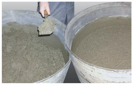
Fig. 7: Concrete before and after addition of plasticising admixture
