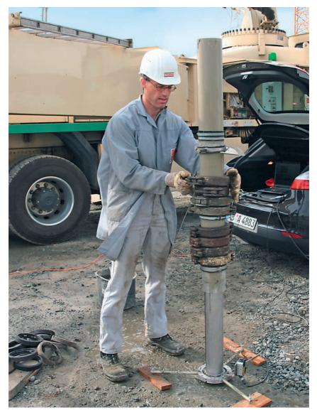
Fig. 34: Measuring the consistency coefficient of freshly-mixed concrete using the Sliding Pipe Rheometer
