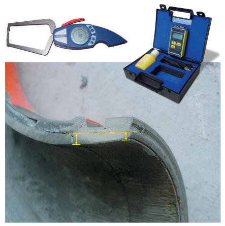
Fig. 32: Measuring pipe wear: wall thickness measuring units for two-layer lines (le.) and single-layer lines (ri.)
