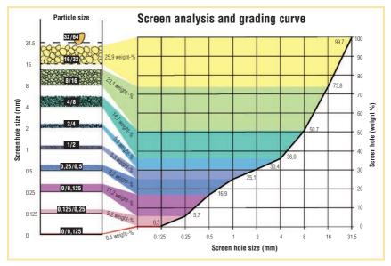
Fig. 3: Sieve analysis and grading curve
