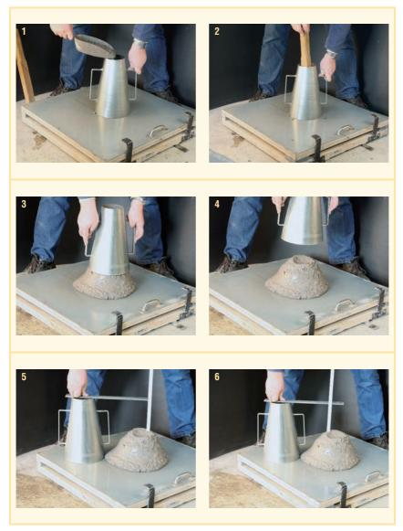
Fig. 11: Measuring slump in accordance with DIN EN 12350-2
