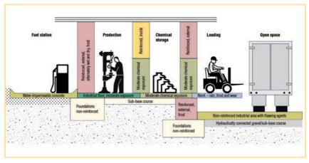
Fig. 14: Exposition classes in the industrial construction\*
